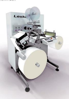
web widths: 280 mm max. unwind dia.: 750 mm max. rewind dia.: up to 440 mm max. speed: 100 m/min
