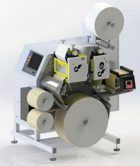
web widths: 280 mm max. unwind dia.: 750 mm
