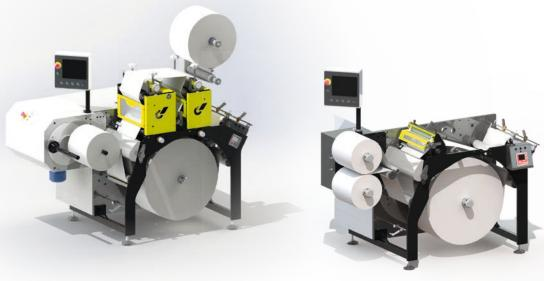
web widths: 280/330 mm max. unwind dia.: 750 mm max. rewind dia.: up to 600 mm max. speed: 220 m/min
